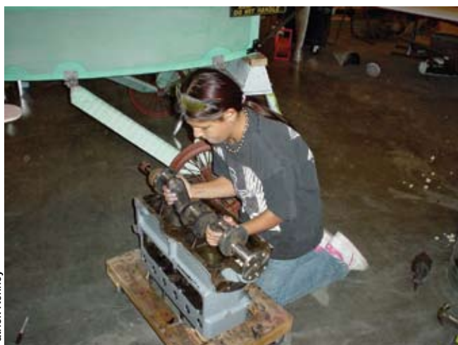
TOP TO BOTTOM: Kimberly Randall honing the cylinder bore on the Ford Model A engine.
