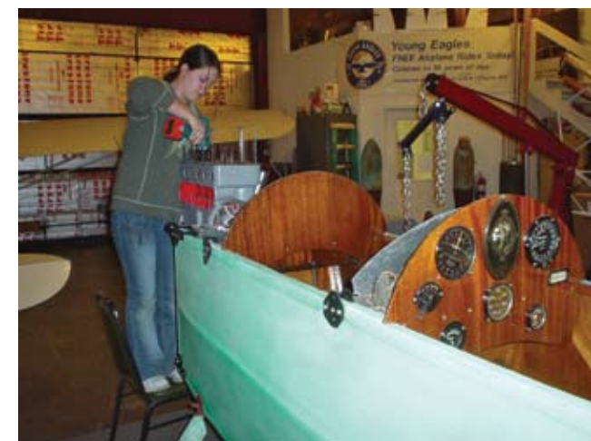
TOP TO BOTTOM: Kimberly Randall sanding the Pietenpol's bottom longeron.
